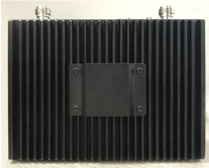
Use 4 screws to fix the other bracket to the repeater's back side.
